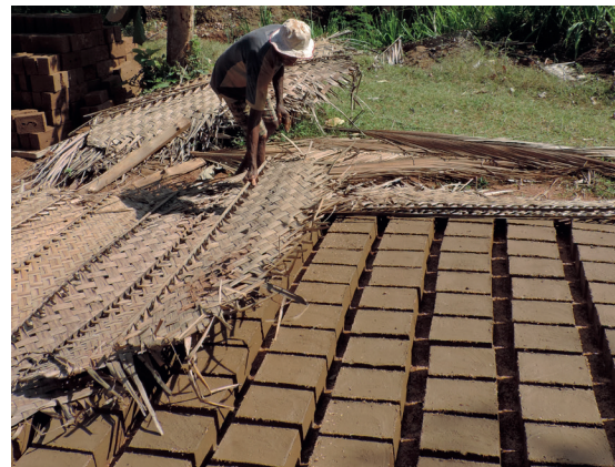
Left: Bricks stacked on top of each other for drying. Right: Bricks left to dry in the sunlight covered with coconut branches to make the drying efficiently and uniformly.
