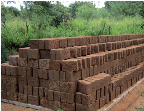
Left: Bricks stacked on top of each other for drying. Right: Bricks left to dry in the sunlight covered with coconut branches to make the drying efficiently and uniformly.
