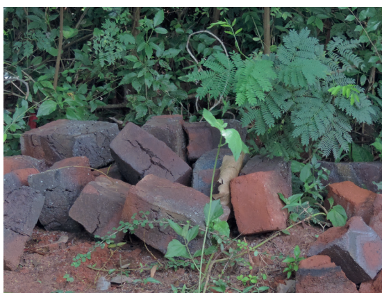
From top left to bottom right: A replica of a temporary kiln facility. A permanent brick kiln facility. Over-fired and under-fired bricks dumped as wastage from a temporary kiln. Interlayer gaps between bricks to be filled with biomass to increase heat circulation and burning inside.
